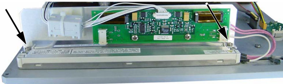
Figure 5-26. Support Bracket for Backlight Driver PCB
