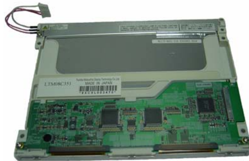
Figure 5-28. LCD Display with Backlight Attached
