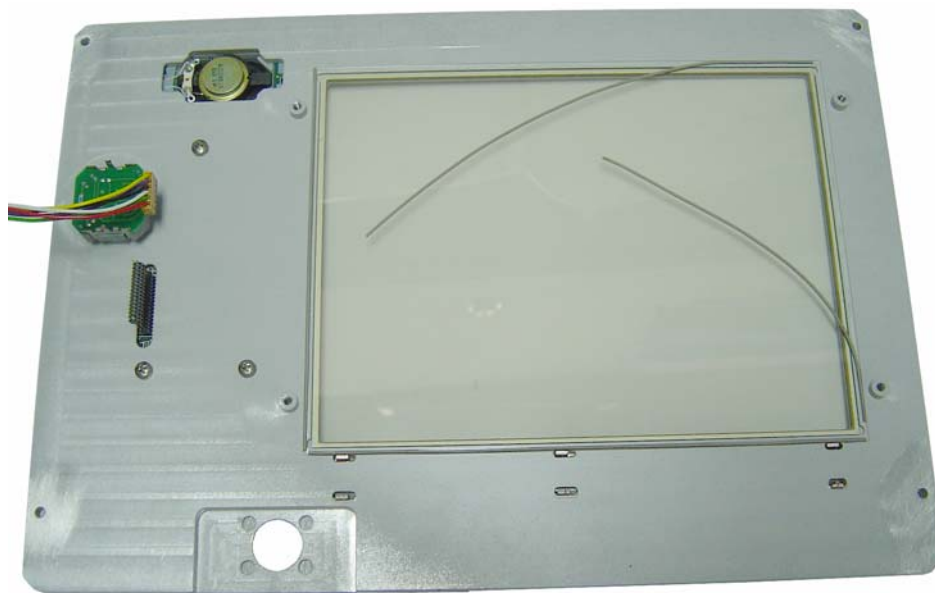
Figure 5-29. Front Panel Gaskets for LCD Display
